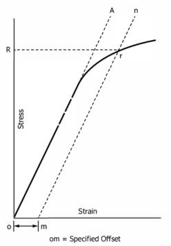
FIG. 9 Stress-strain Diagram for Determination of Yield Strength by Offset Method
