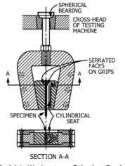
FIG. A4.1 Wedge-type Gripping Device
