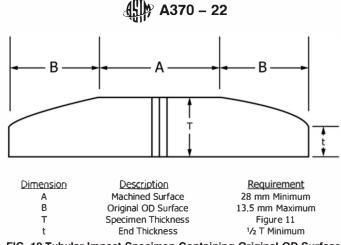
FIG. 12 Tubular Impact Specimen Containing Original OD Surface
