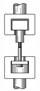
FIG. A3.1 Tension Testing Full-size Bolt
