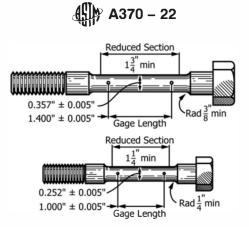
Note 1-Metric equivalent: 1 in. = 25.4 mm. FIG. A3.4 Examples of Small Size Specimens Proportional to Standard 2-in. Gauge Length Specimen
