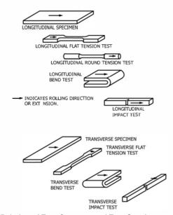
FIG. 1 Relation of Test Coupons and Test Specimens to Rolling Direction or Extension (Applicable to General Wrought Products)
