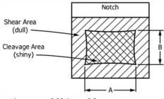
NOTE 1-Measure average dimensions A and B to the nearest 0.02 in. or 0.5 mm. NOTE 2-Determine the percent shear fracture using Table 8 or Table 9. FIG. 13 Determination of Percent Shear Fracture
