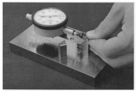
FIG. 16 Lateral Expansion Gauge for Charpy Impact Specimens
