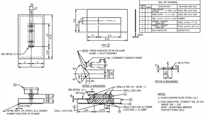
FIG. 17 Assembly and Details for Lateral Expansion Gauge
