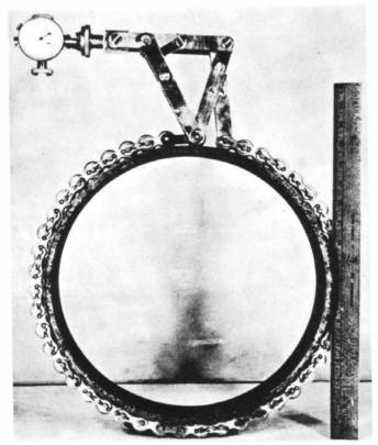
FIG. A2.8 Roller Chain Type Extensometer, Clamped
