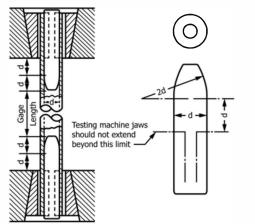
FIG. A2.1 Metal Plugs for Testing Tubular Specimens, Proper Location of Plugs in Specimen and of Specimen in Heads of Testing Machine
