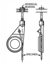
FIG. A4.2 Snubbing-type Gripping Device
