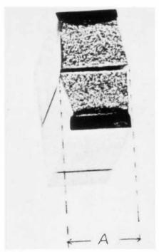
FIG. 15 Halves of Broken Charpy V-notch Impact Specimen Joined for Measurement of Lateral Expansion, Dimension A
