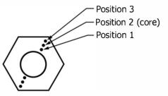
FIG. A3.7 Hardness Test Indentation Locations
