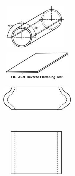
FIG. A2.10 Crush Test Specimen
