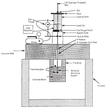
FIG. 3 Typical Fire Test Setup
