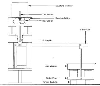
FIG. 2 Tension Creep Test Arrangement Using a Dead Weight
