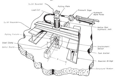
FIG. 1 Tension Creep Test Arrangement
