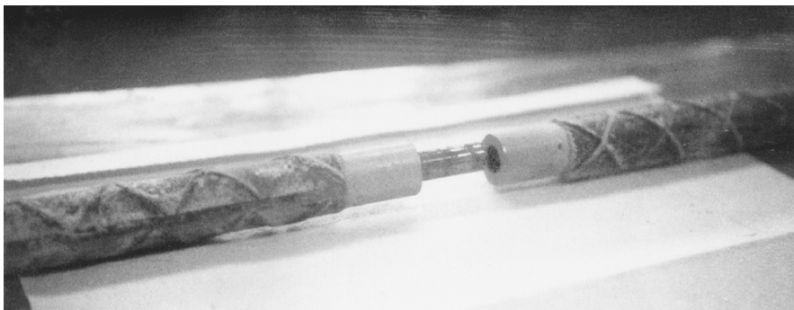
Figure 41 The RE-bar at the joint assembly. Slip joint detail of the RE-bar for tension testing of concrete cylinders. The overall length of the finished RE-bar assembly = 75 cm or 30 in. The slip joint at the center is to be lightly lubricated. The ends of each of the RE-bars at the joint are to be machined to just remove the deformations for a length of about 2.5 cm or 1 in.
