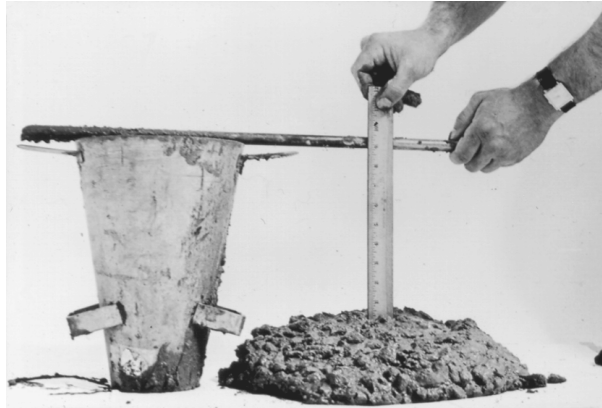
Figure 20 Demonstration on use of a slump cone: (top) a low slump and (bottom) a high slump. (From the Canadian Portland Cement Association. With permission.)
