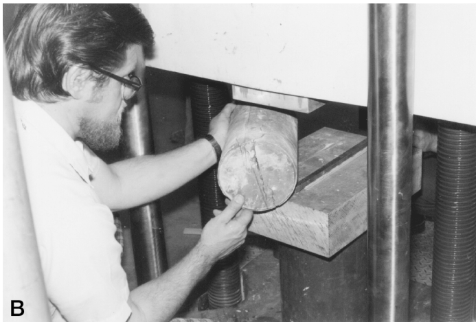
Figure 36 (Top) Specimen being positioned in the testing machine. (Bottom) After the concrete specimen was loaded to failure and removed from the test apparatus with fracture indicated.
