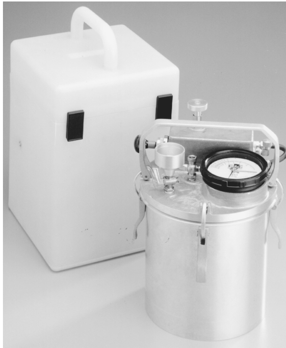
Figure 23 Type B air meter. (Courtesy of ELE International, Inc., Soiltest Products Division, Lake Bluff, IL.)
