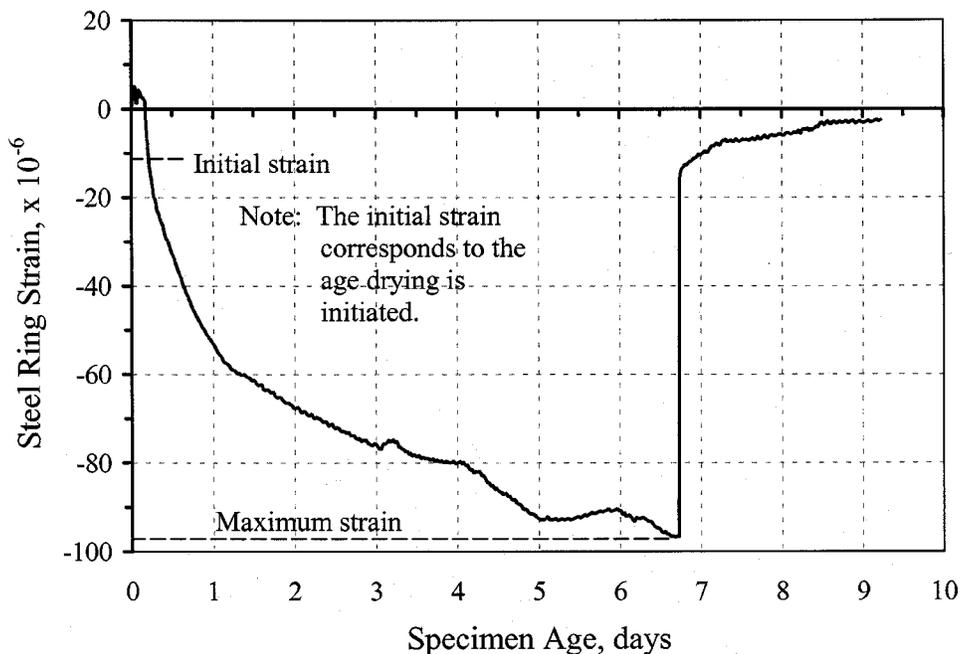
FIG. 2 Steel ring strain versus specimen age.
