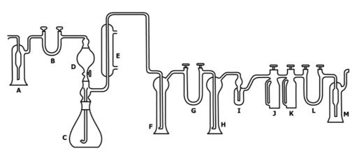
FIG. 1 Apparatus for Carbon Dioxide Analysis
