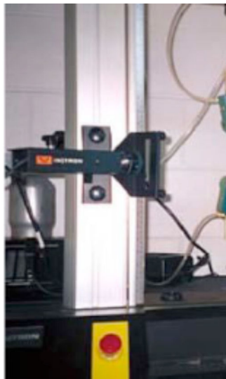
a. Photograph of Video Extensometer
