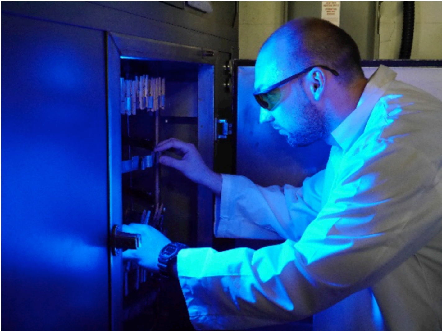
Photograph #4: sample set up in a Xenon arc unit
