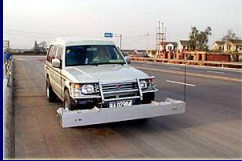
Dynatest RSP 5051 Mk II "L5.2c" in Jiangsu, China. (5 Laser, 2 gia tốc kế)
